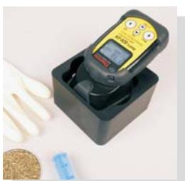
The RadEye B20 / B20-ER can be set to display the net count rate by automatically subtracting the stored background data. See the manual for details.
